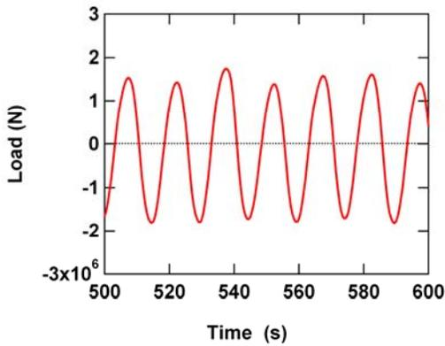
Figure 6. Vertical force (Design 2 – 13.1m wave height)
