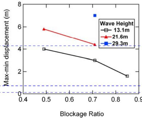
**Figure 9. Centerwell wave height vs. blockage ratio**
