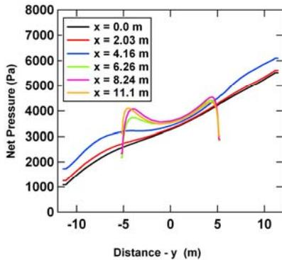
Figure 7. Load distribution on the centerwell plate at a time of maximum load, Design 2
